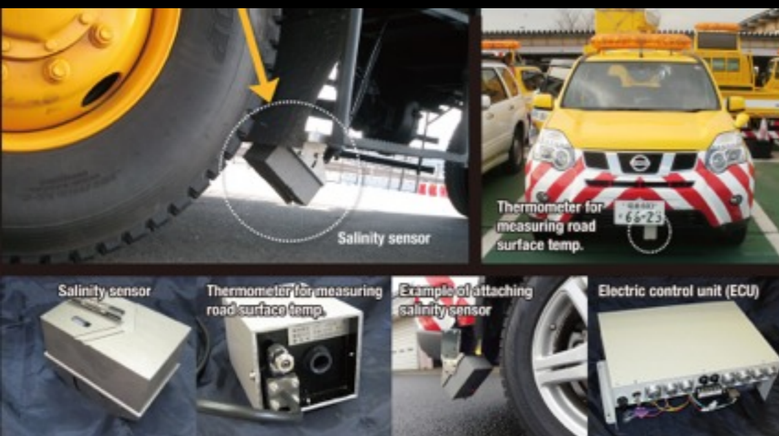
Configuration of the onboard salinity measurement system
